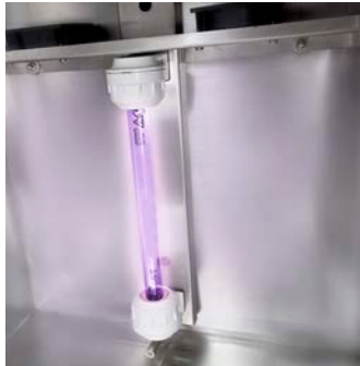
Air UV recirculation system in the chamber
