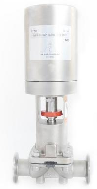
inside the valve. The diaphragm separates the lower valve body cavity from the inner cavity of the upper valve cover, so that the valve stem, the valve flap and the like located above the diaphragm are not corroded by the medium, the packing sealing structure is omitted. The compressed air is used to drive the drive screw to move the spool up and down, and at the same time pull the diaphragm up and down to close and open. This model has adjustable minimum flow regulator.
