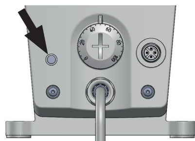
Fig. 18: Signal LED A signal LED is located on the fore side of the pump; it indicates operating states and errors
